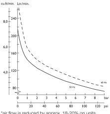
\*air flow is reduced by approx. 18-20% on units with dryer
